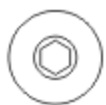
Socket button head collar screw 半圓頭內六角軸套螺絲 (M3x10mm) x 4
