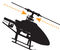
Without SAFE® technology, the swashplate briefly steers against the rotation but then goes back to neutral when the helicopter is not moved anymore.
